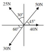
(b) Determine the magnitude direction and position of resultant force of the force system given in figure with reference to point A.
